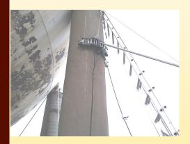
The standard Bracelet is used with a pole and rope system to inspect sphere legs
